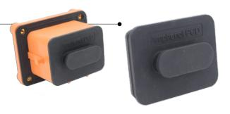
MINI MSD M XXX / F Shell type: M: Plug F: Receptacle Fuse rating current: **XXX:** 080, 100, 125, 160, 200, 250, 315, 350, 400 (Unit: AMP) 000: No fuse needed, can directly use the terminal Fuse brand (this applies to plugs): /: Bussmann (by default) 1: Other brands (TBD) Flange mounted type (this applies to sockets): **F:** Front mounted R: Rear mounted
